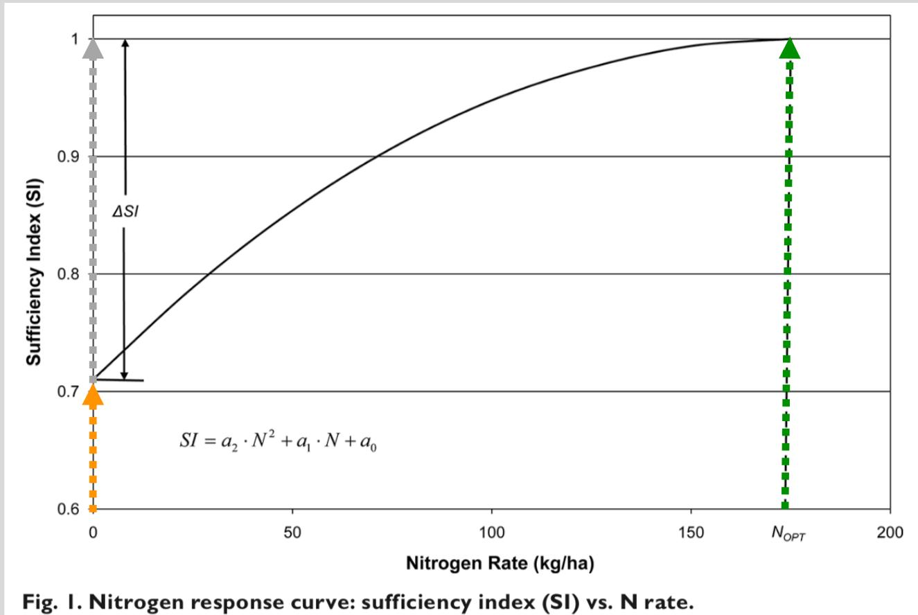
Fig. 1. Nitrogen response curve: sufficiency index (SI) vs. N rate.
